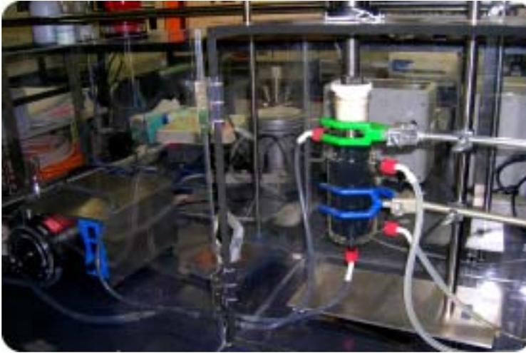
Photo 1. Peristaltic tube pump (left) and sonorod in flow vessel. The latters are contained in a plastic box for suppressing excessive noise.
