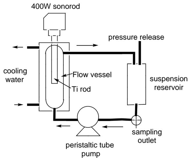
**Fig. 1.** Schematic illustration of an ultrasonication set-up. A 300 mL separatory funnel was used as the reservoir of circulating suspension (see also Photos 1 and 2).
