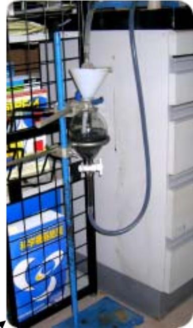
Photo 2. Reservoir for suspension-colloid is placed below the flow vessel to prevent overflowing through the loose contact between sonorod and PFTE joint.
